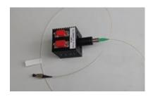
Thanks to their low losses and transmission up to 5.5  $\mu$ m, our fluoride fibers are particularly adapted to ICL/QCL pigtailing.
